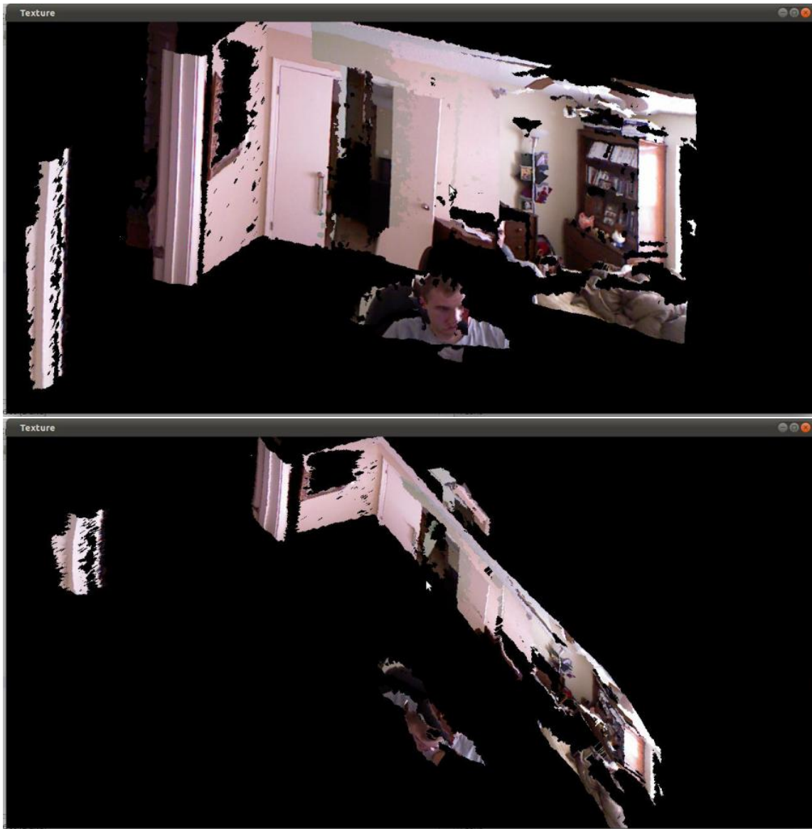
Figure 21: Combined model from two different angles, showing improved visibility.
